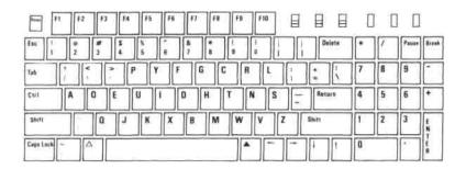
Fig. 4-2 (b) Keyboard switch is set to ALT (The simplified keyboard)
